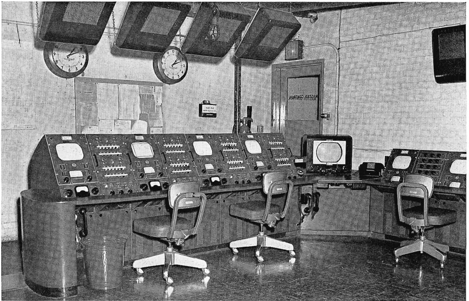
FIG. 31. Front view of the WOR-TV Master Control Switching Console which consists of facilities for switching six incoming circuits to four outgoing channels.
