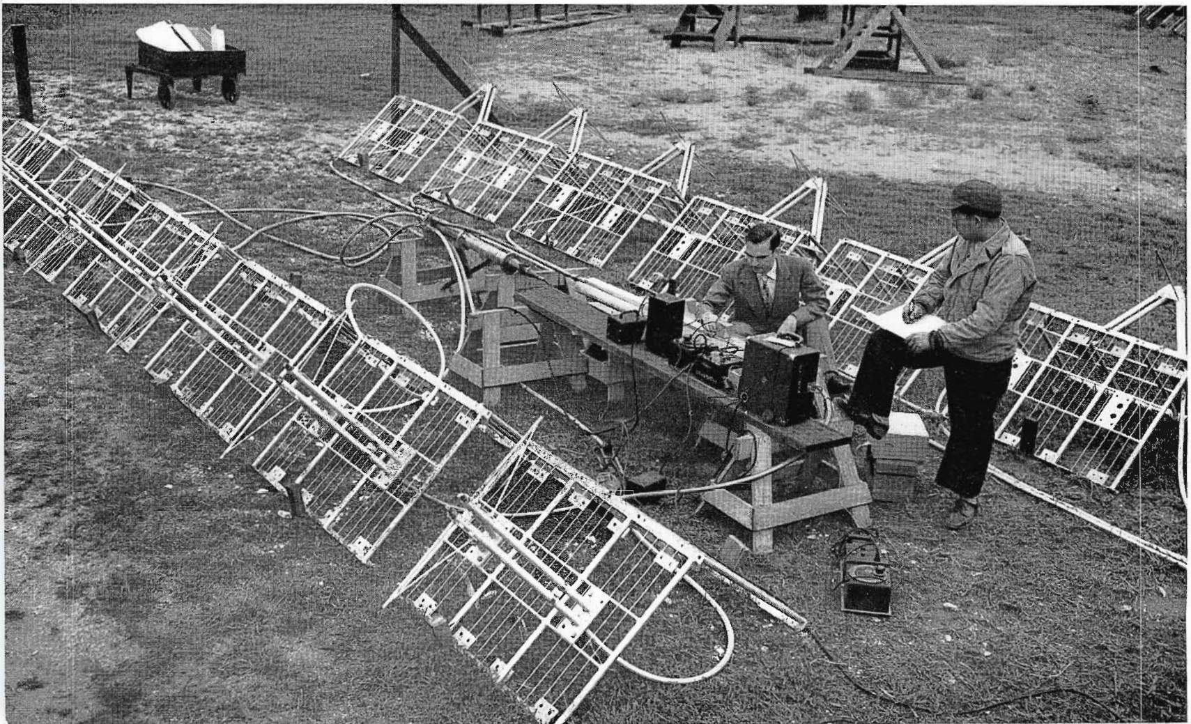
FIG. 3 (below). At Camden, RCA Engineer Howard King at right and assistant are shown making impedance measurements on the Channel No. 7 antenna elements.
