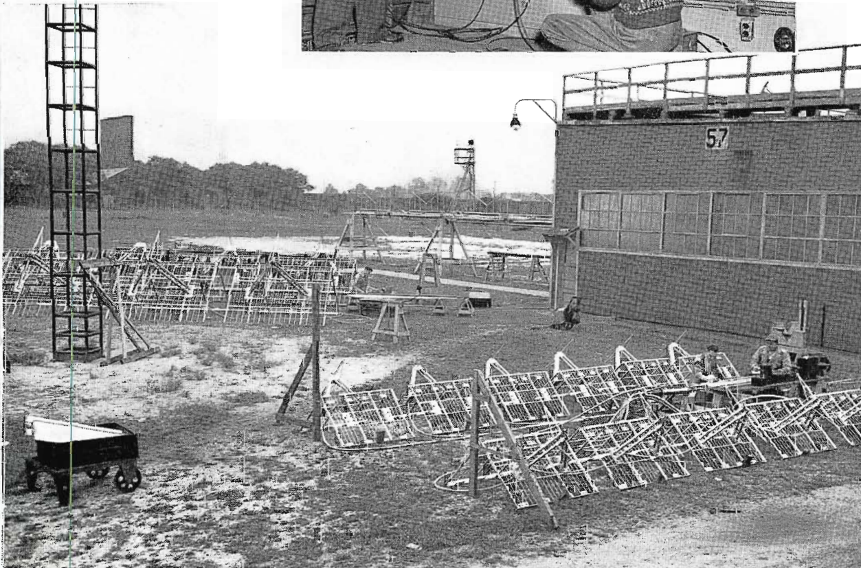
FIG. 6. Partial view of the engineering field laboratory showing the Channel No. 7 antenna under test in the foreground and Channel No. 5 antenna in background. Near building, Channel No. 4 Super Turnstile is visible.
