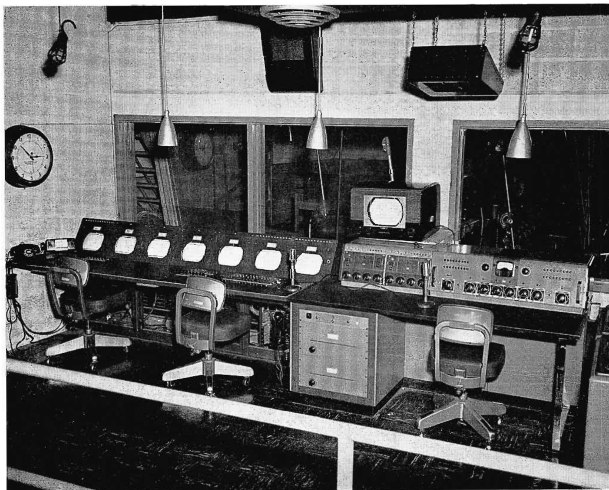
FIG. 11. View of Control Room "A" showing the WOR-TV Program Director's Console at left and the Audio Console at right.
