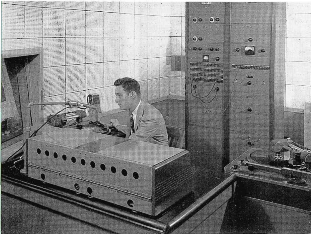
FIG. 2. The Master Control room includes RCA Consolette, 70 series turntables, recorder attachments and equipment racks. Announcer Jack McKee is at the console controls.
