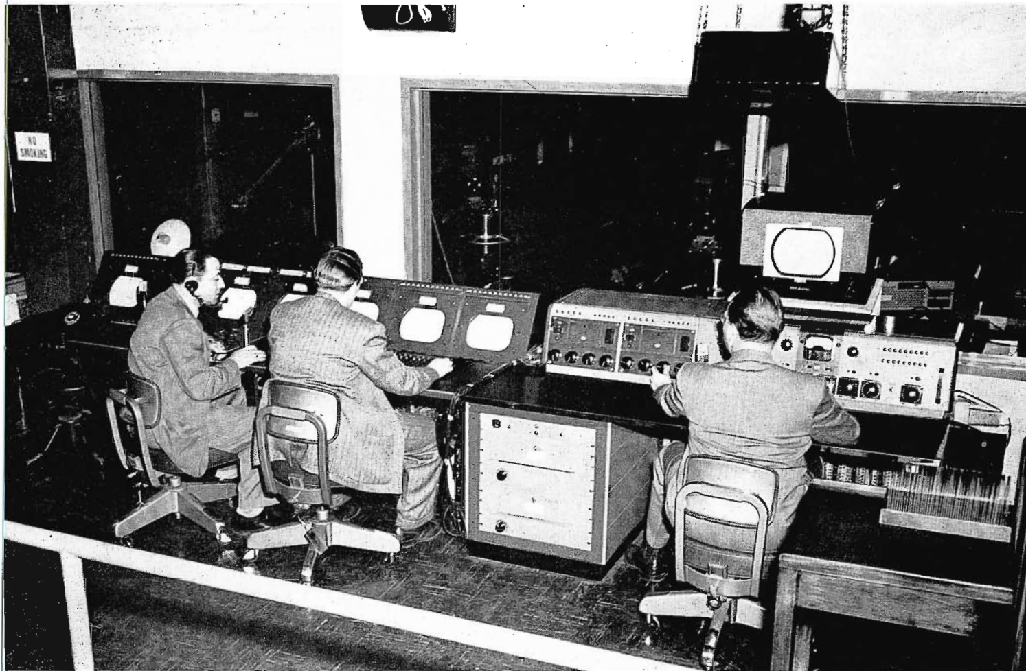
FIG. 12 (below). Studio Control Room "B" during program operation (Program Director at left watches seven monitors; Preview 1, Cameras 1, 2, 3 and 4, Preview 2 and Line Monitor). Video Switcher sits at director's right and audio engineer at audio mixing controls.
